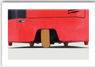
3-pivot design, with better stacking stability
